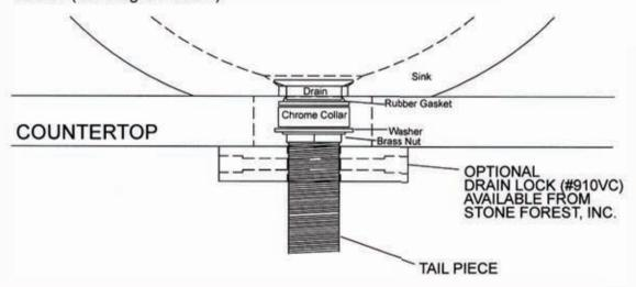
Required drain use 9054D Grid Drain or 9058D Lift and Turn Drain. This can be supplied by Stone Forest at your request in select finishes.
