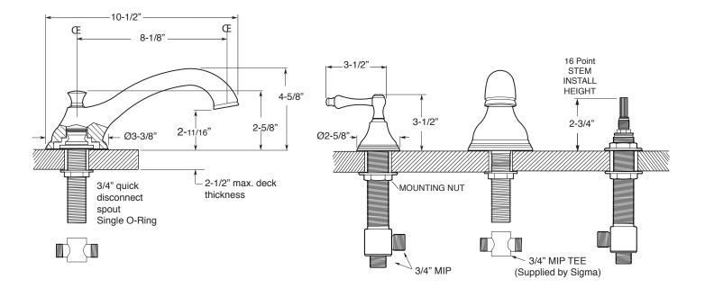
NOTE: Spout and valves install through 1-1/4" diameter holes. Plumber to provide 3/4" supply lines to valves
