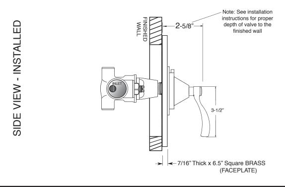
All-thread Metric Holding Tube 1/2" NPT Outlets
