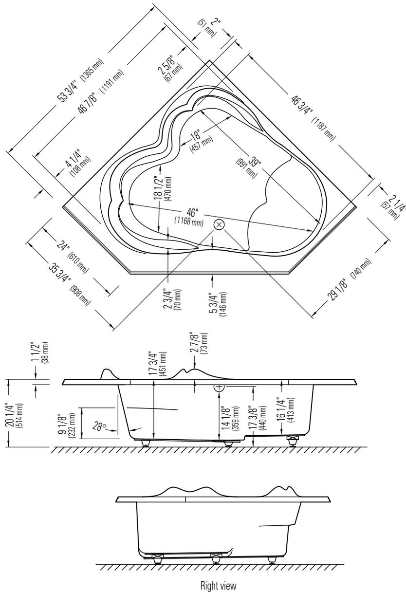
\*A bathtub fitted with back jets can cause the pump to protrude by approximately 3" from the overall dimension.
