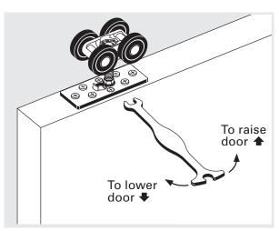
Use adjusting wrench supplied to adjust door clearance
